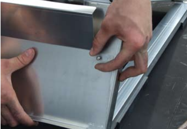
Start screw in existing top right hole
