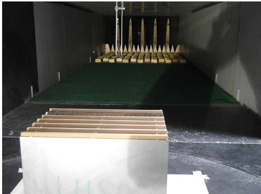
**Figure 1.2:** Wind tunnel model of the type building with the system ilzoeasy and with covered edge zones
